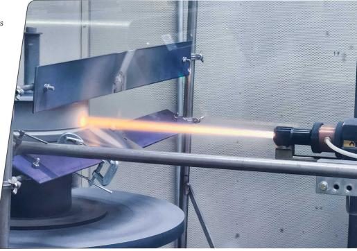
Metco atmospheric plasma spray system, a Thermach twinwire arc system and Linde/Praxair HVOF equipment.
