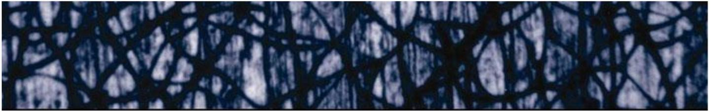
**ULTRAKOAT:** The ultimate coating for Blow Molding. Nano-crystalline deposit of diamond-like particles co-deposited with hard Nickel Alloy. UltraKoat offers superior corrosion/erosion resistance while improving distribution of material with a permanently lubricious surface. It is normally applied from .0002 to .0005 thick. The uniform metallic surface is permanent.
